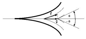
Figure 3. Speed of skeleton formation by fire front quenching. The original object outline is denoted by bold lines, different discrete stages of the fire-front development are shown dotted.  $\vec{t} = d\underline{y}/ds_y$  is the tangent to the fire-front,  $2\theta$  is the angle of the meeting fronts. The skeleton formation speed  $\|\vec{v}\|$  will therefore be proportional to  $1/\sin(\theta/2)$ .
