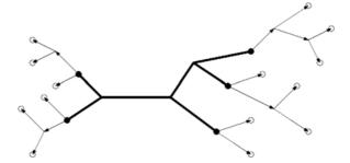
Figure 7. Definition of a skeletal core playing the role of the topological skeleton for objects with disk topology. The edges shown in bold on this hypothetical skeletal graph build the core declared to be undeletable by assigning a significance measure to them exceeding some selected threshold. The roots of the tree-components are denoted by filled circles; the imposed partial ordering from the roots to the leaves (empty circles) is indicated by the arrow direction on the deletable edges.
