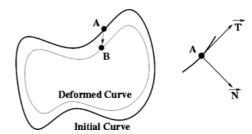
Figure 5. The deformation of an initial curve is described by the displacement of each point in the tangential and normal directions.
